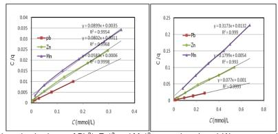
Figure 4. Langmuir adsorption isotherm of Pb<sup>2+</sup>, Zn<sup>+2</sup> and Mn<sup>+2</sup> on apatite mineral (A) mono-metal and (B) ternary-metal
